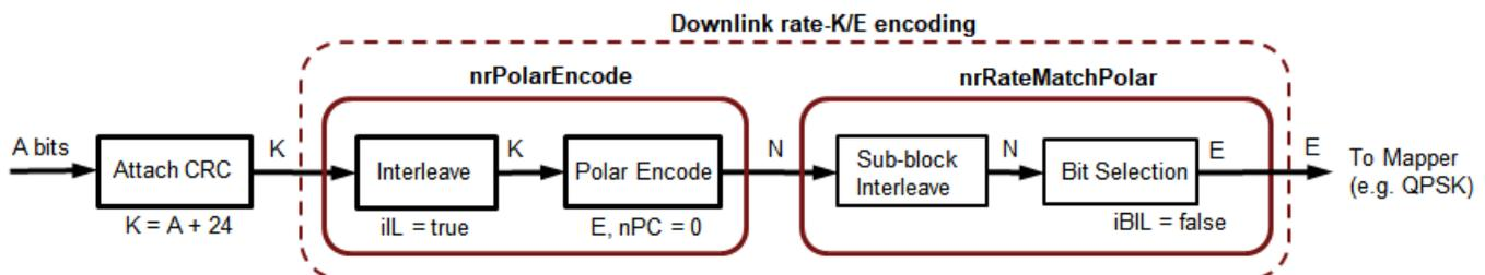
For the downlink, the input bits are interleaved prior to polar encoding. The CRC bits appended at the end of the information bits are thus distributed for the CA-Polar scheme. This interleaving is not specified for the uplink.
